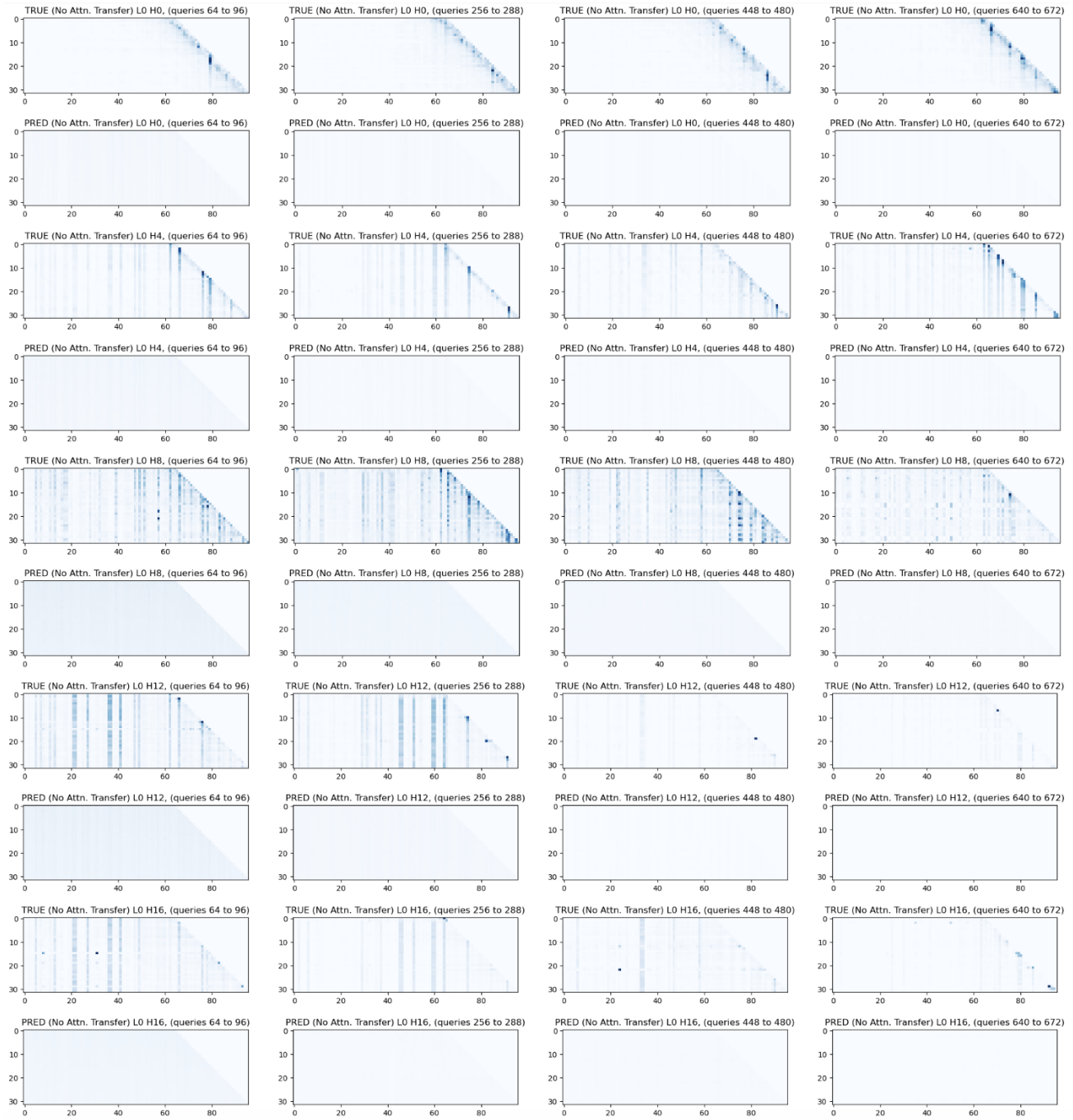
Figure 4. Linear attention (PRED) and softmax attention (TRUE) weights for exp learned feature map, without attention transfer.
