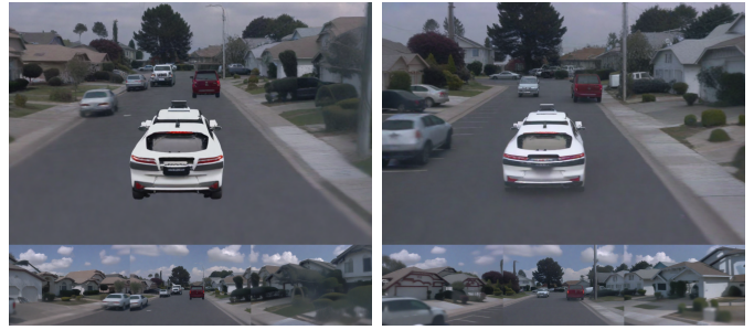
Fig. 5. Composability with Dynamic Actors. We simulate driving trajectories in a residential street scenes for a Waymo-representative [3] sensor stack. From bottom to top, we show a third-person view of the ego capture vehicle followed by a set of rendered front cameras. Both columns correspond to a different timestamp of the same traffic configurations + fully generated scene & asset models. The second vehicle is hidden behind the corner in the first frame.
