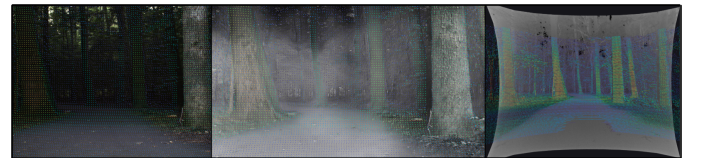
Fig. 6: Multi-modal data from the M2P2 dataset, showcasing spatial and temporal alignment in a low-light, off-road forest environment. LiDAR point cloud overlaid on RGB image (left), reconstructed event frame at the trigger’s falling edge (middle), and thermal image (right).
