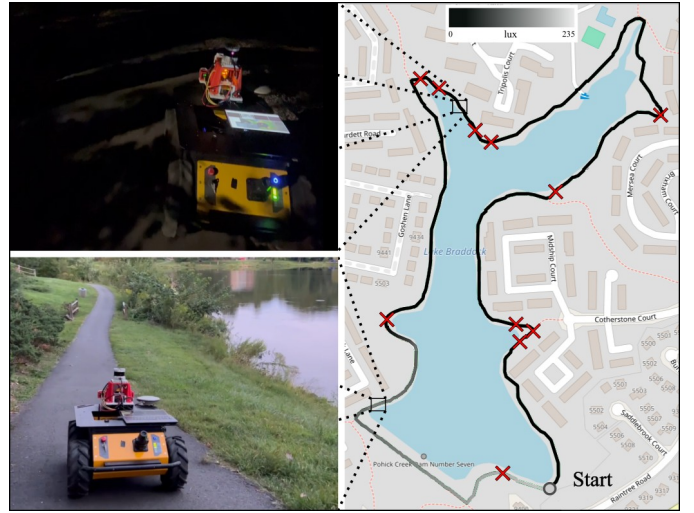
Fig. 9: Autonomous Navigation around a 3.6 km Trail with a BC model and Thermal Input: Lighting conditions drops from 255 lx at the beginning (light gray on the path, lower right) to 0 lx (black, upper left). 11 interventions (red crosses) are necessary to correct the robot when going off-course.
