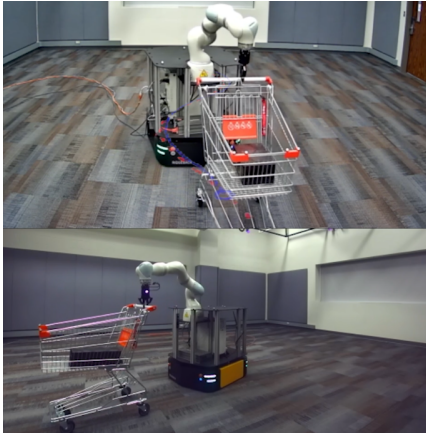
Fig. 3. Picture of the MM pushing the heavy shopping cart during a curved trajectory tracking experiment.
