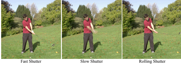
Figure 2. Physics-grounded temporal augmentation. We synthesize low-rate videos from 240 FPS sources using sharp capture, exposure integration, and rolling-shutter simulation.
