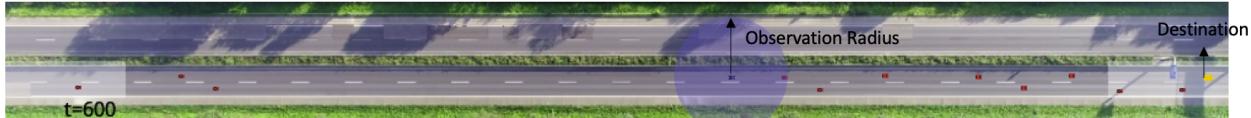
Figure 9: (Figure 5 in (Liu et al., 2023)) The Highway Driving (HighD) environment. The ego car is blue, other cars are red. The ego car can only observe the things within the region (marked by blue). The goal is to drive the ego car to the destination (in yellow) without going off-road, colliding with other cars, or violating time limits and other constraints (e.g., speed and distance to other vehicles).
