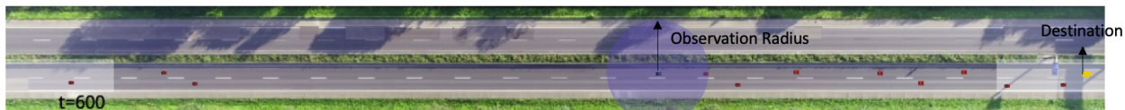
Figure 9: (Figure 5 in (Liu et al., 2023)) The Highway Driving (HighD) environment. The ego car is blue, other cars are red. The ego car can only observe the things within the region (marked by blue). The goal is to drive the ego car to the destination (in yellow) without going off-road, colliding with other cars, or violating time limits and other constraints (e.g., speed and distance to other vehicles).
