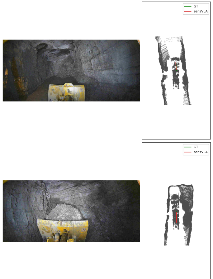
Fig. 2: Qualitative predictions on two validation frames (loading approach). On the BEV, the ground-truth 2 s ego-path is drawn in green and sensVLA’s prediction in red.
