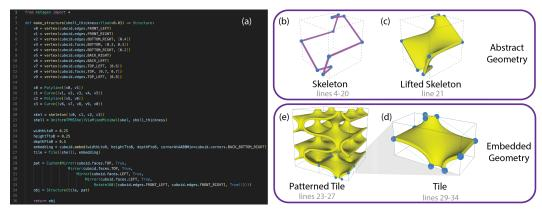
Figure 1: A MetaDSL program (a) and illustrations of each construction stage (clockwise): (b) build a 1D skeleton relative to an abstract convex polytope CP – here, a cuboid; (c) specify a lifting procedure from 1D to 3D; (d) embed the CP in  $\mathbb{R}^3$  to create a tile, and execute the lifting procedure to create our final geometry; and finally, (e) tessellate the tile according to the specified pattern.
