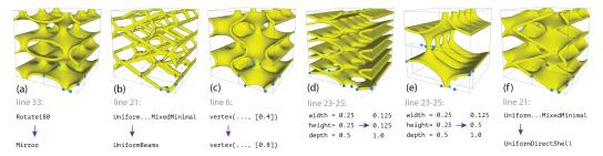
Figure 2: We illustrate the expressive power of MetaDSL by showing six different structures that all stem from the program shown in Figure 1(a). Each one is produced by changing a single aspect of the original program, as detailed below each structure.
