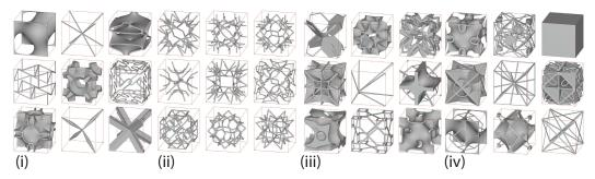
Figure 3: Assortment of metamaterials in MetaDB, illustrating four creation modes: (i) hand-authored seeds, (ii) generated models, (iii) type-enabled mutations, and (iv) LLM-augmented hybrids.
