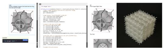
Figure 4: Reconstruction: (Left) Generating a metamaterial program from an input image enables incorporating designs from literature, sketches, and nature. (Right) 3D printed design.
