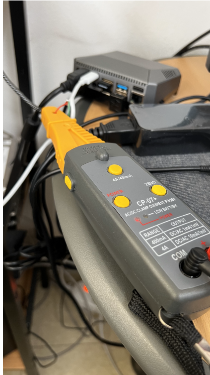
Figure 12: A realistic environment for estimating energy consumption. Using a current probe with \pm 1.5\% accuracy resolution, the amount of current in a USB power cable was measured.
