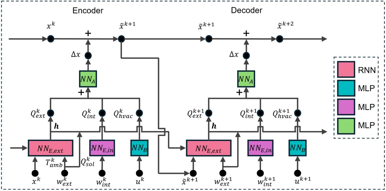
Figure 1. Physics-Informed Building Dynamic Model used in BESTOpt
