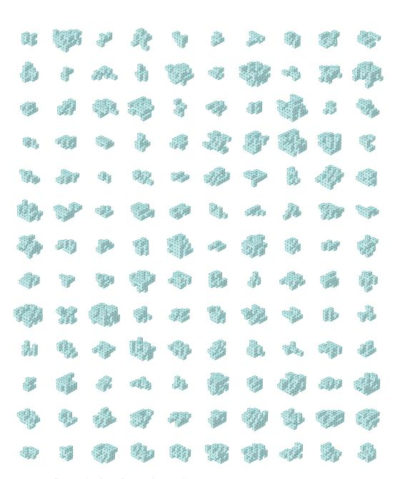
Figure 11: **Generalization of pretrained universal controller.** Randomly sampled morphologies from the top 50% of performers in generation 0 of zero-shot evolution. The universal controller successfully controls these diverse, previously unseen robot designs, demonstrating effective generalization across morphologies.
