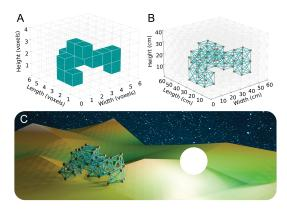
Figure 3: Genotype to phenotype. Designs are encoded by voxel genotype (A), which is expressed as a spring-mass phenotype (B), and evaluated in a differentiable environment (C). The springs (teal lines in B and C) and masses (orange spheres) are motorized and sensorized, respectively.
