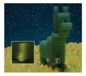
Figure 13: **Scaling morphology.** The embarrassingly parallel nature of the co-design pipeline allows the compute required to simulate 1024 robots with up to 1648 springs (i.e. a single GPU) to be redistributed for a single robot with 1,115,157 springs.
