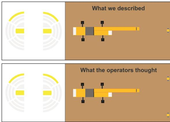
Figure 16: The first concept of proximity warning was understood differently by the operators when the obstacle is exactly in the front or behind the cabin. However, this way of thinking was not wrong either, since if there are two obstacles, where one is in the left side and the another one is on the right side of the cabin, the visualization will then look the same.
