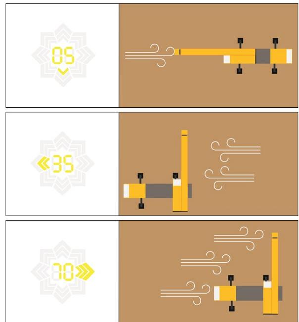
Figure 11: The arrows in the left side images and the wind icon in the right side images represent both wind direction and wind force. The wind direction is always shown depending on where the cabin is facing. The numbers in the center indicate the estimated wind speed.
