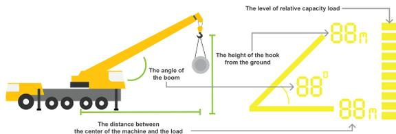
Figure 13: The meaning for each component in the concept for showing the relative load capacity.
