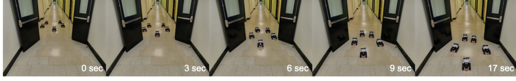
(a) A team of five physical robots with a circular formation navigates through a narrow doorway in a hallway.
