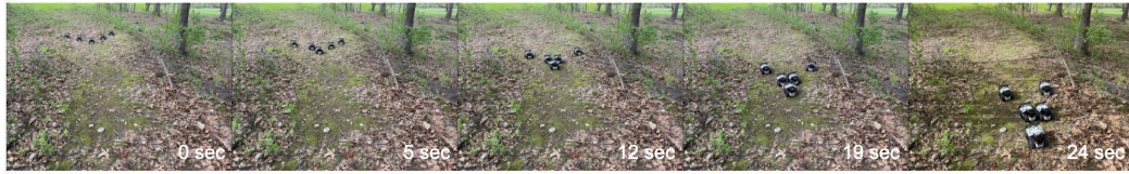
(b) A team of five robots with a wedge formation navigates through a forest-like environment characterized by narrow corridors, scattered trees, and surrounding obstacles.
