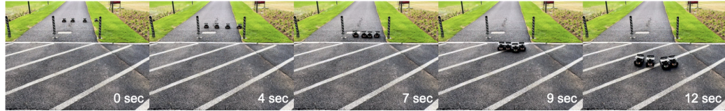
(c) A team of four robots in a line formation navigates through a narrow pathway, where robots access is restricted by two sticks marking the boundaries.
