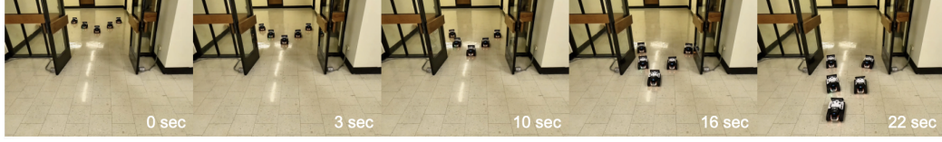
(b) A team of five robots with a wedge formation navigates through a narrow exit.
