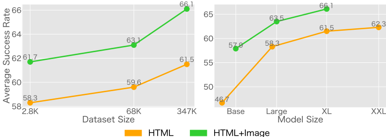
Figure 5: Average success rate of WebGUM with different dataset (left) and model sizes (right). X-axis is a logarithmic scale. As for both HTML and multimodal models, we could observe the scaling effect: the larger the dataset and model size are, the higher the success rates are. Surprisingly, our approach outperforms previous SL state-of-the-art (48.4% by Gur et al. (2022)) more than 9.9% even with 2.8K-episode dataset (about 25% of the previous dataset curated by Liu et al. (2018)). See Appendix F for further details.
