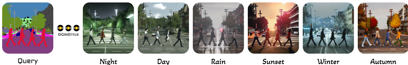
Figure 1. Crossing domain boundaries with DGInStyle. We propose a data-centric generative pipeline for domain generalization. It is derived from Stable Diffusion and augmented with a novel high-precision style-preserving semantic control. DGInStyle combines semantic masks (Query) with style prompts (e.g., Night or Rain) to generate training data for semantic segmentation networks with widely varying appearance. DGInStyle achieves state-of-the-art semantic segmentation across domains in autonomous driving.
