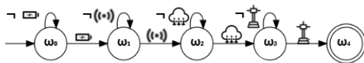
Figure 3: DFA for Mountain Car Collection . Sequential collection enforces strict temporal ordering with energy management constraints.
