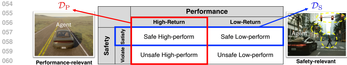
Figure 1: Illustrative example of safety–performance dual demonstrations. We consider two types of demonstrations, \mathcal{D}_S and \mathcal{D}_P , where \mathcal{D}_S comprises constraint-abiding safe behaviors that may exhibit suboptimal performance, while \mathcal{D}_P consists of high performance behaviors that may violate underlying safety constraints.
