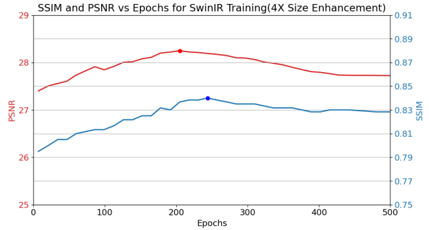
Figure 5. Training progression for SwinIR instance in HDL-SAM, particularly highlighting its effectiveness in achieving a 4\times up-scaling task. The graph presents the average PSNR (depicted in red) and SSIM (represented in blue color) throughout a training period of 500 epochs.
