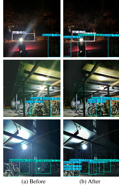
Figure 13: Object detection with flare-corrupted and flare-removed images. Flares can obscure objects such as bicycles and motorcycles, making them undetectable.
