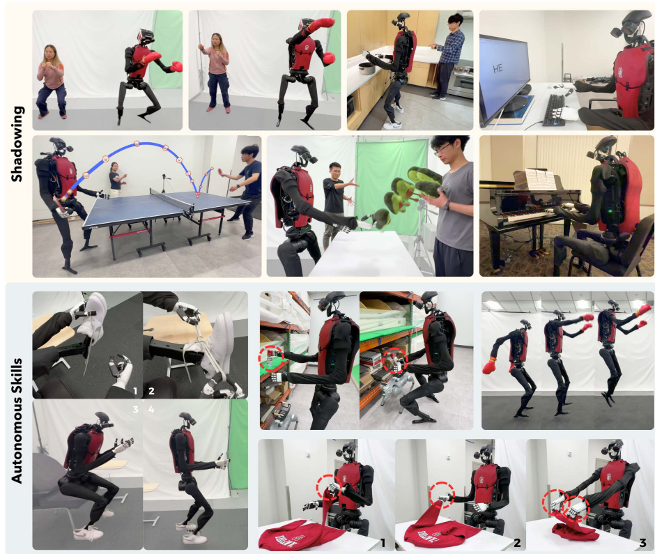
Figure 1: We present a full-stack system for humanoid robots to learn motion and autonomous skills from human data. Our system enables robots to shadow fast, diverse motions from a human operator, including boxing and playing table tennis, and to learn autonomous skills like wearing a shoe, folding clothes, and jumping high.
