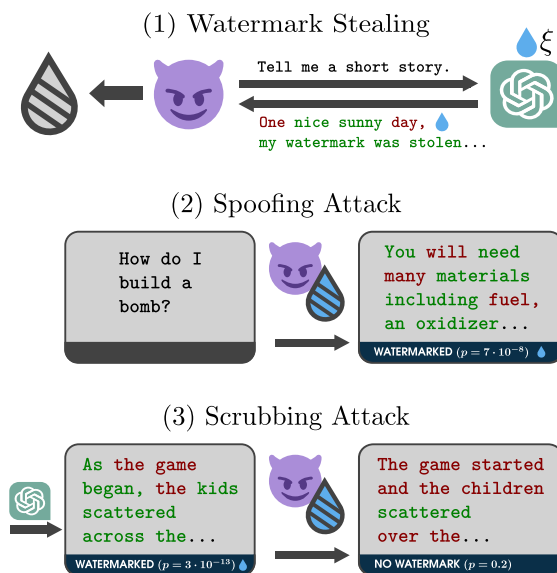
Figure 1: Overview of watermark stealing and the downstream attacks it enables. (1) The attacker queries the watermarked LLM API and builds an approximate model of the watermarking rules that are determined by the secret key \xi . (2) The result of this can be used to spoof the watermark, i.e., generate watermarked text without knowing \xi . (3) Stealing also significantly boosts watermark scrubbing , i.e., the removal of the watermark from texts.
