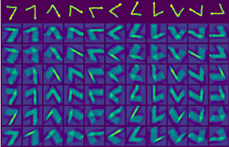
Figure 2: Rotation equivariance of a randomly initialized SE(2) Chebyshev convolutional layer. From left to right shows different rotations of an input (top row) and the activations for different slices of \theta \in [0, \pi] in the graph (bottom 6 rows). A rotation of an input image followed by Chebyshev convolution is equivalent to first convolution followed by a planar rotation in each \theta slice and a roll in the \theta -axis.
