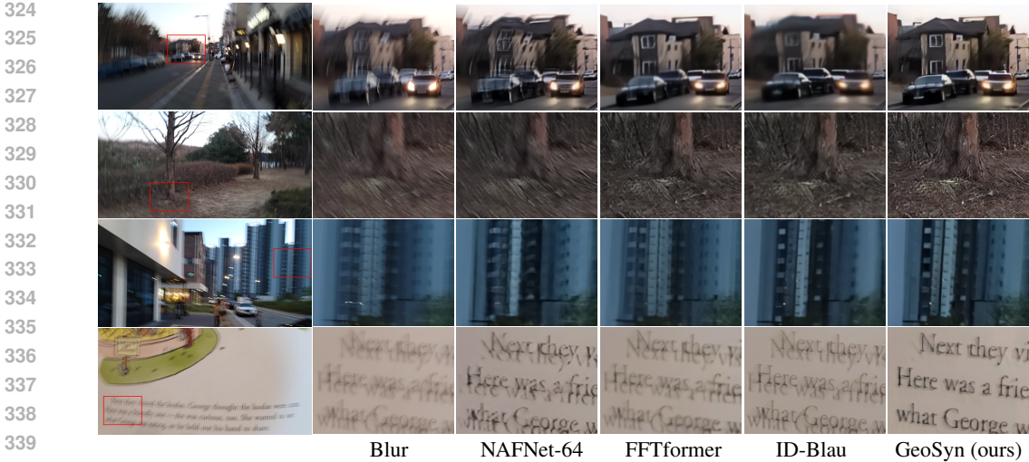
Figure 7: Qualitative comparison results on real-world blur images. NAFNet is used for all methods. Our blur synthesizer produces sharper and artifact-free results compared to state-of-the-art methods.
