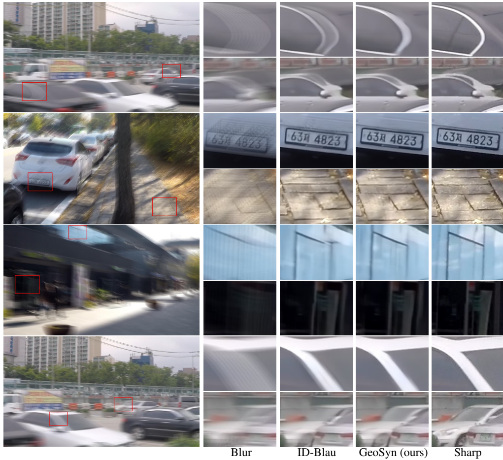
1490 Figure 12: Qualitative results on GoPro (Nah et al., 2017). All models are trained with GoPro and 1491 are based on MIMO-UNet (Cho et al., 2021). 1492 1493 1494 1495 1496 1497 1498 1499 1500 1501 1502 1503 1504 1505 1506 1507 1508 1509 1510 1511
