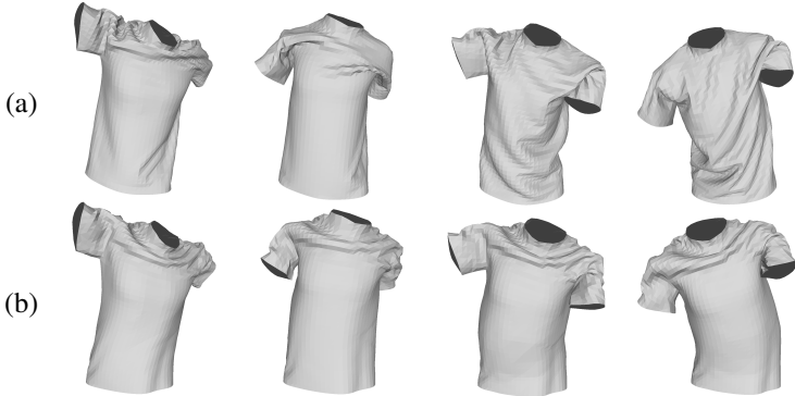
Figure 3: (a) The ground truth cloth and (b) skinning the cloth using a fixed tetrahedral embedding. Note how poorly this naive embedding of the cloth into the KDSM matches the ground truth (especially as compared to a more sophisticated embedding using our plastic deformation as shown in Figure 4).
