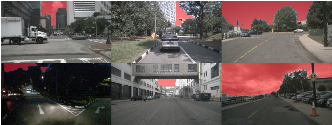
Figure 16: Visualization of sky segmentation results from the LISA model on the nuScenes dataset. Leveraging a language-guided segmentation model, we achieved highly accurate sky segmentation, even in challenging conditions such as complex and low-light scenes.
