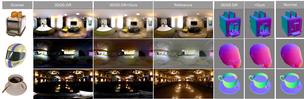
Figure 10: Qualitative comparisons of HDR reconstruction and normal reconstruction by 3DGS-DR (Ye et al., 2024) and our proposed method. The better performance of HDR and normal reconstruction means better reflective object reconstruction performance.
