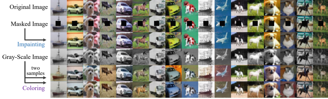
Figure 6: The visualization of image recuperation in the inpainting and coloring tasks. The experiment is performed by Algorithm 4 from [32], which iteratively mixes the image with a reference image created by adding and removing noise at time t with t decreasing from T to 0.
