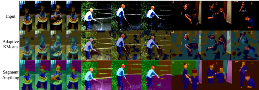
Figure 3: Adaptive discrete visualization. Objects that exhibit similar visual appearance across frames should map to consistent clusters. We compare an adaptive K-means variant (visualized with a reduced number of clusters for clarity) and Segment Anything (SAM) as adaptive clustering front-ends.
