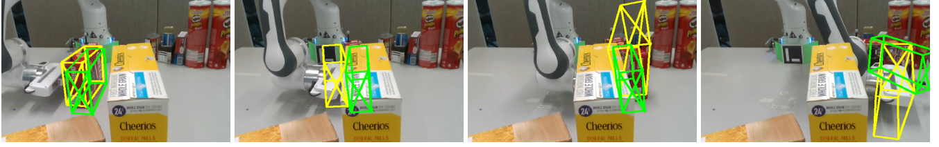
Fig. 1. Robot pushing a Cheezit object (red box) among cluttering objects. Images are from the tracking camera. Estimated object pose of our proposed method (PBPf) is shown as green wireframe box. The estimated object pose from a vision-only pose estimation system (DOPE) is shown as a yellow wireframe box. (Please note wireframe boxes are overlaid on the images as post-processing. While the green box appears on top of the obstacle/robot hand in some images, this is only an artefact of the way we overlay these wireframe boxes. The pose estimates are in fact behind the obstacle/robot hand in these instances, close to the actual object pose. Please also see the accompanying video.)
