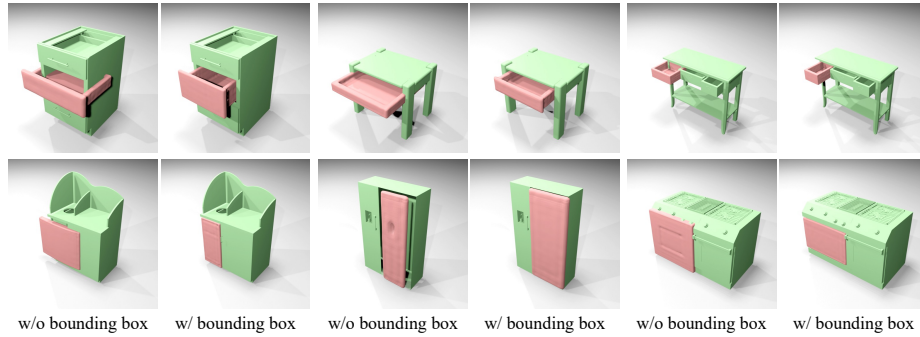
Fig. 9: Comparison between whether or not using the bounding box as an additional condition. Incorporating the bounding box beside the point cloud enhances the fit of the generated part to the given object.
