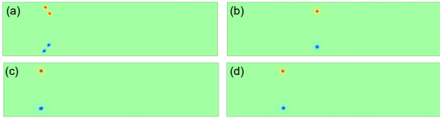
Fig. 10. 2D Leapfrog Marathon. The vortex pairs simulated by LFM remain separate after a round trip. (a) LFM (b) LFM without leapfrog method (c) PFM (d) NFM
