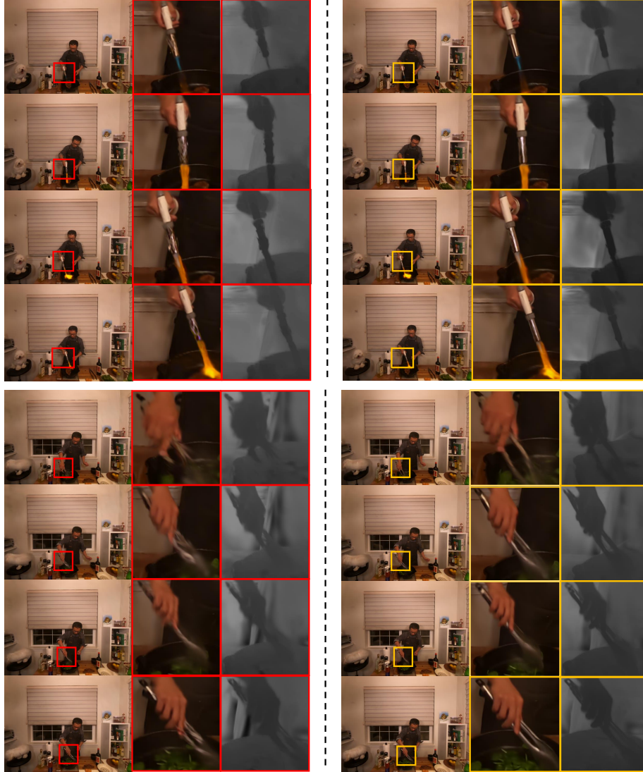
Figure 11: Qualitative comparisons on DyNeRF dataset (Li et al., 2022). The left column shows the novel view rendered images and depth maps of a 4D Gaussian method Yang et al. (2023c), which suffers from artifacts in the dynamic regions. The right column shows the results of the same method while optimized with our flow supervision during training.
