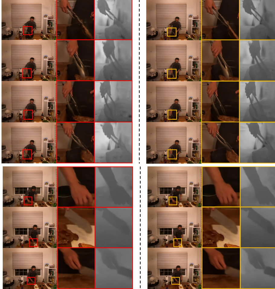
Figure 12: Qualitative comparisons on DyNeRF dataset Li et al. (2022). The left column shows the novel view rendered images and depth maps of a 4D Gaussian method (Yang et al., 2023c). While The right column shows the results of the same method while optimized with our flow supervision during training.
