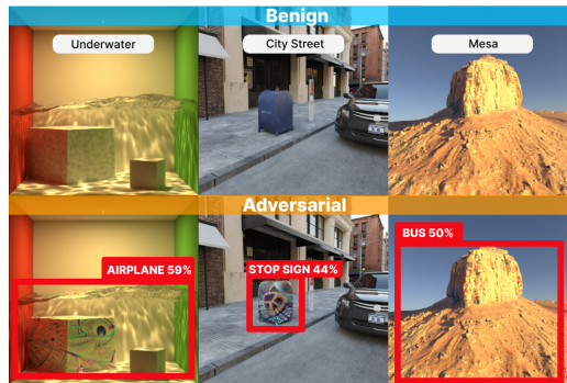
Fig. 1: REVAMP enables users to easily perturb textures on objects in realistic scenes (top row), inducing incorrect detection of an underwater cube as an airplane, a mailbox on a city street as a stop sign, and a mesa as a bus (bottom row).
