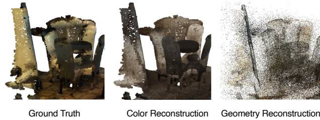
Figure 4: The visualization of reconstruction results from Point-GCC. Note that we decrease the point size in geometry reconstruction to avoid the block from noisy points.
