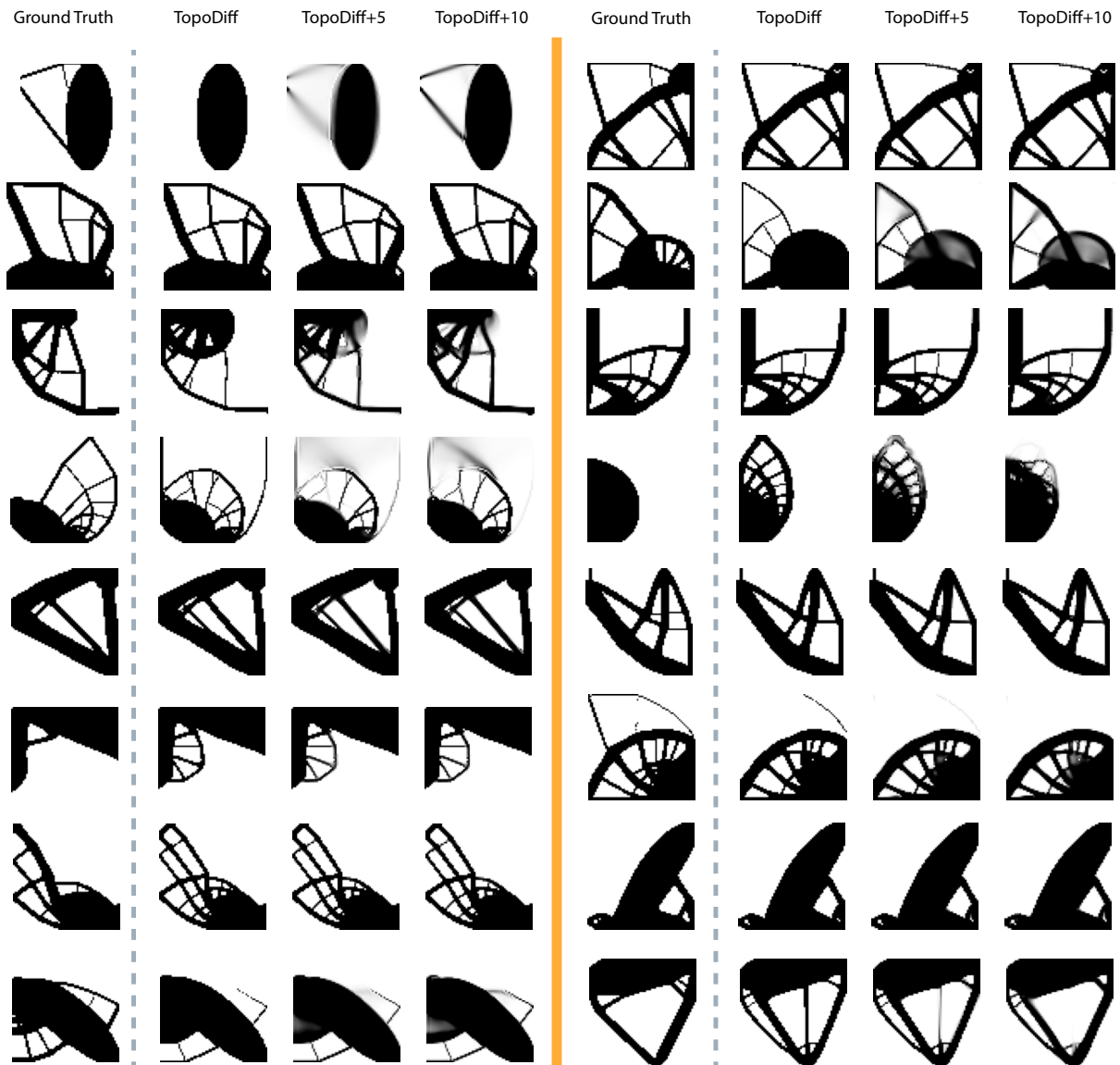
Figure 10: Visualization of the effect of direct optimization on samples generated by TopoDiff. The first column of each set of images shows the ground truth, the next column shows the samples generated by TopoDiff, and the two columns that follow show the effects of 5 and 10 steps of direct optimization on the samples respectively. These samples are from the 64x64 test set.
