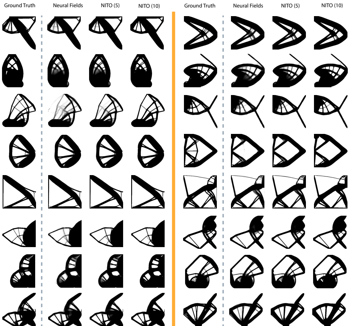
Figure 9: Visualization of the effect of direct optimization on samples generated by neural fields. The first column of each set of images shows the ground truth, the next column shows the raw predictions from neural fields, and the two columns that follow show the effects of 5 and 10 steps of direct optimization on the samples respectively. These samples are from the 256x256 test set.
