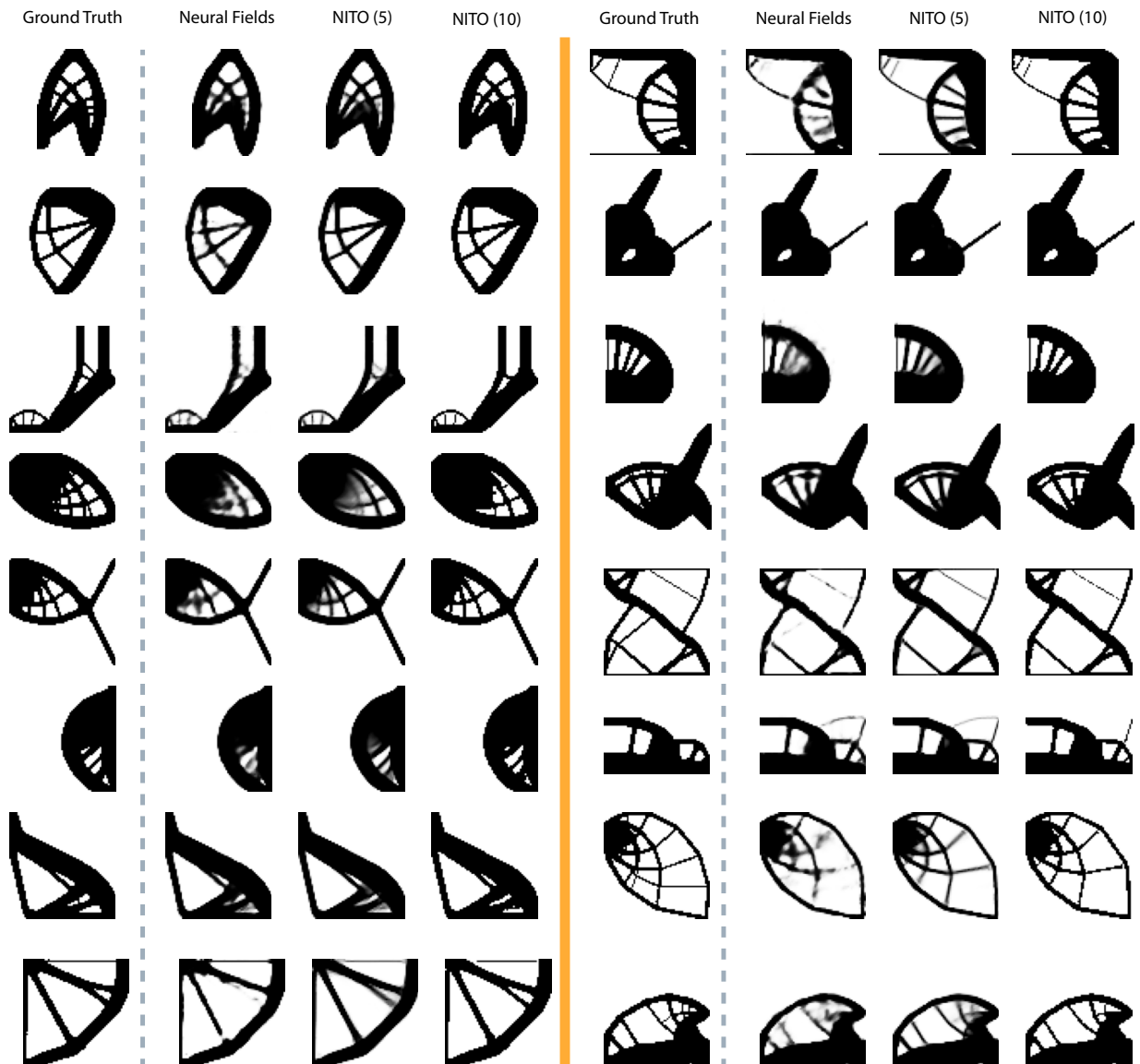
Figure 8: Visualization of the effect of direct optimization on samples generated by neural fields. The first column of each set of images shows the ground truth, the next column shows the raw predictions from neural fields, and the two columns that follow show the effects of 5 and 10 steps of direct optimization on the samples respectively. These samples are from the 64x64 test set.
