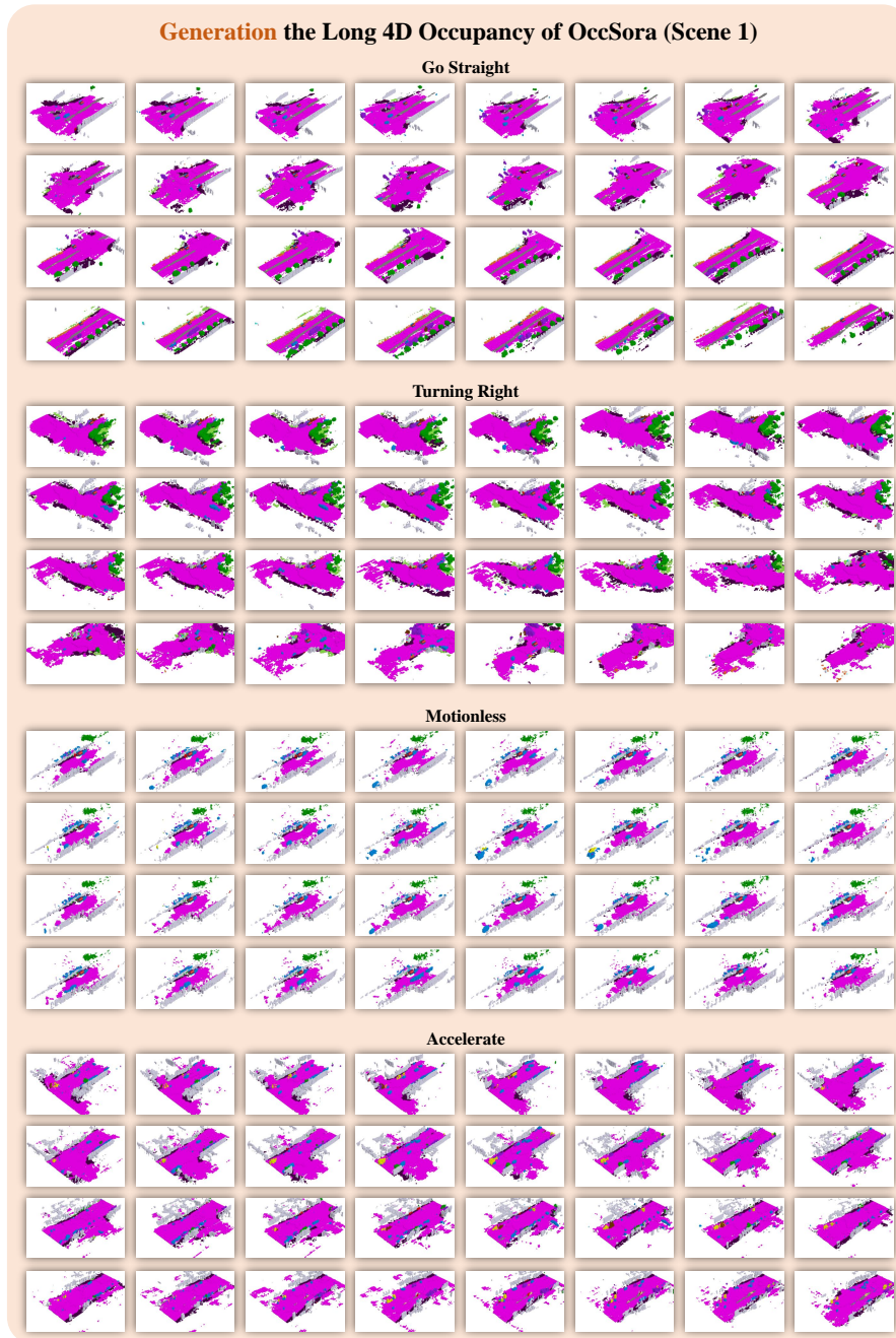
Figure 17: The ability to generate long time-series 4D occupancy under different trajectory controls. From top to bottom, we present long-term continuous scenes generated under four types of ego vehicle trajectories: Go Straight, Turning Right, Motionless, and Accelerate.
