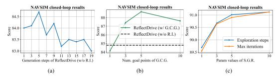
Figure 4: Ablation on (a) the number of generation steps for *ReflectDrive* (w/o R.I.), (b) the number of goal points for Goal-Conditioned Generation (G.C.G.), and (c) the numbers of exploration steps as well as max iterations for Safety-Guided Regeneration (S.G.R.).
