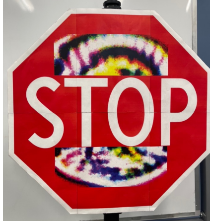
Figure 7: FTE-Y5 H1 + H2 with TV loss STOP signs attack generation, which is printed on ledger-size papers.
