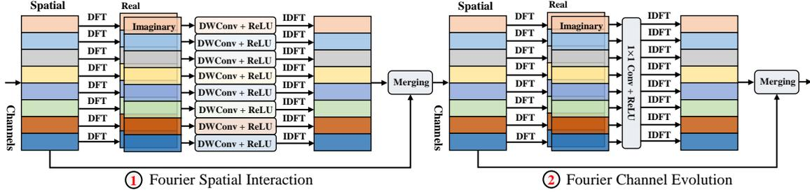
Figure 4. Details of the Fourier Prior Embedded Block. The FPE Block follows the same global modeling rule “spatial interaction + channel evolution” but is with new designs: Fourier spatial interaction modeling and Fourier channel evolution.
