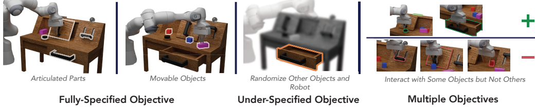
Figure 3: Experiment Setup. In the CALVIN simulator [30], we propose four experimental setups designed to showcase DynaGuide and its advantages over other steering approaches. First, we test performance with high quality outcome observations as guidance conditions ( Fully-Specified Objective ). Next, we reduce the guidance condition quality by randomizing robot states and other states not relevant to the target object ( Underspecified Objective ). Finally, we look at how we can guide the base policy in complex ways, including achieving multiple behaviors and avoiding behaviors ( Multiple Objectives ).
