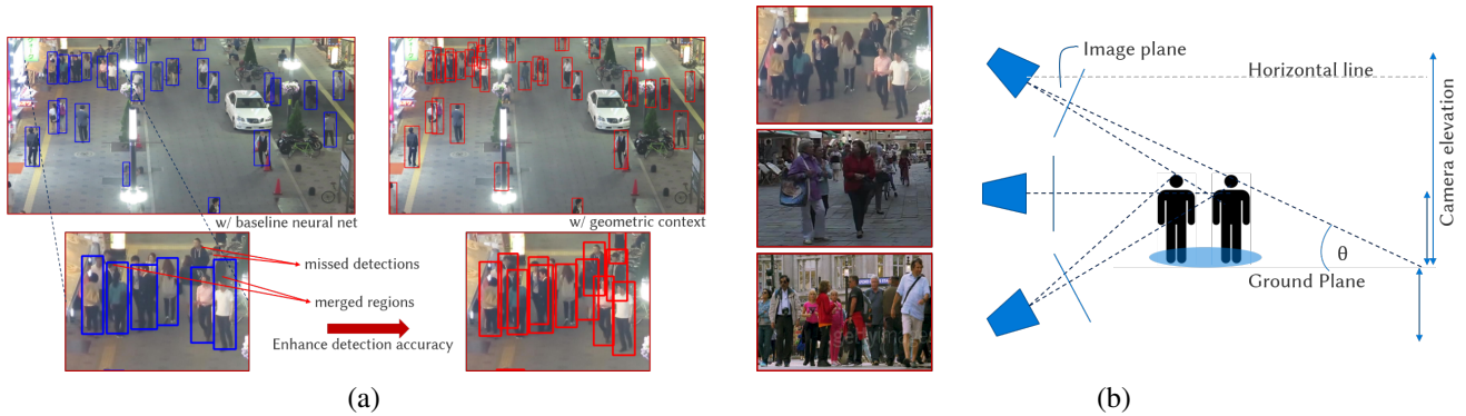
Fig. 1: Standard detectors under-perform in crowded scenes. We factor in scene geometry to recover occluded instances. Right : The occlusion pattern of nearby objects in the image depends on the camera viewpoint w.r.t. the ground plane in 3D.
