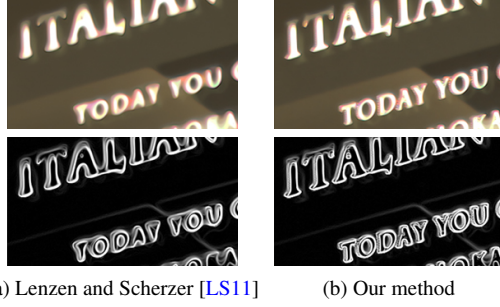
Figure 8: Comparison of blur removal methods. (Left) output HDR image. (Right) gradient image. (b) preserves corners better than (a).
