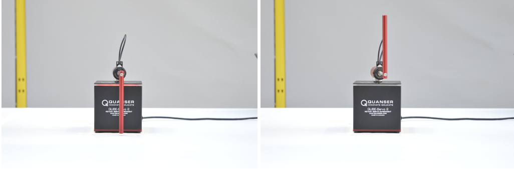
Figure 16: Hardware setup . The Furuta pendulum starts from a downward position (left) and is swung upright. Then, we use a state-feedback controller to balance the pole (right).
