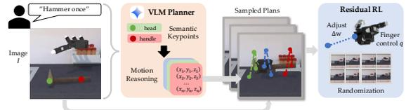
**Fig. 1:** Overview of our method: a VLM generates hand and object keypoint trajectories from a language command and scene image. A low-level residual RL policy is trained to track these trajectories in simulation.
