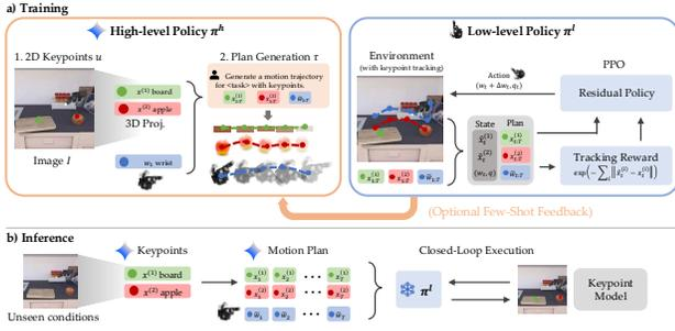
**Fig. 2:** a) Training: a high-level VLM predicts 3D keypoint plans, which a low-level policy learns to track via RL. b) Inference: new plans are generated by the VLM, which are executed by the frozen low-level policy.
