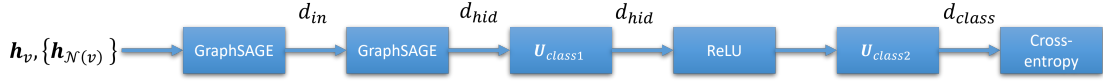
Figure 4: Architecture of the GraphSAGE backbone. \mathbf{h}_v : the node attribute of the central node v . \{\mathbf{h}_{N(v)}\} the node attribute set of the central node v 's neighbours. d_{in} : the dimension of inputs. d_{hid} : the dimension of hidden layers. d_{class} : the number of classes. \mathbf{U}_{class1} \in \mathbb{R}^{d_{hid} \times d_{hid}} . \mathbf{U}_{class2} \in \mathbb{R}^{d_{class} \times d_{hid}} .
