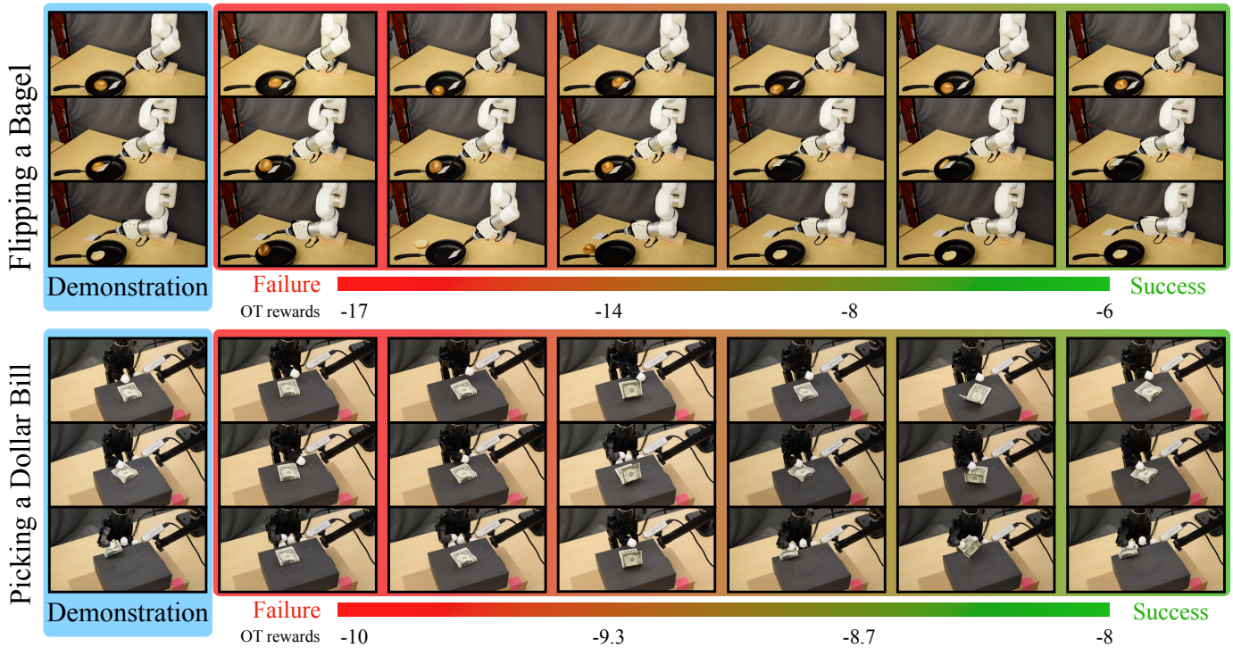
Fig. 5: An analysis of the values of OT rewards for different trajectories with respect to a given expert demonstration. The leftmost column depicts the visual demonstration, while the other columns each depict a trajectory rollout. Trajectories are sorted in increasing order of OT rewards from left to right. Raw OT scores can be visualized using the red-to-green color map.
