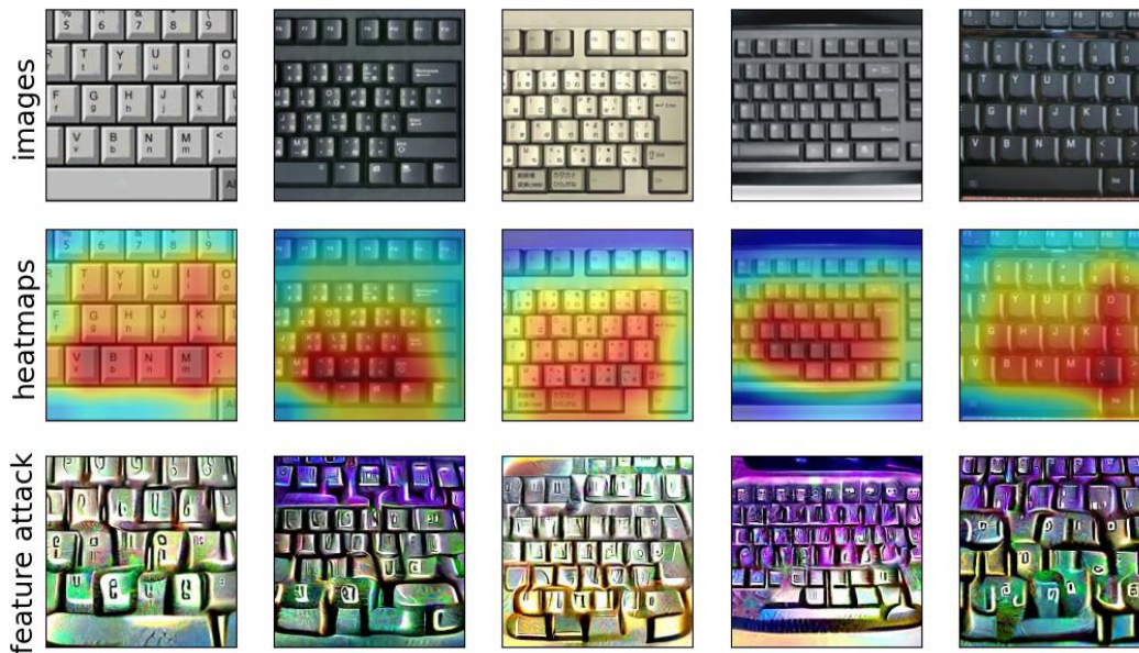
Figure 42: Visualization of feature 325 for class space bar (class index: 810 ). Train accuracy using Standard Resnet-50: 59.043% . Drop in accuracy when gaussian noise is added to the highlighted (red) regions: -46.154% .
