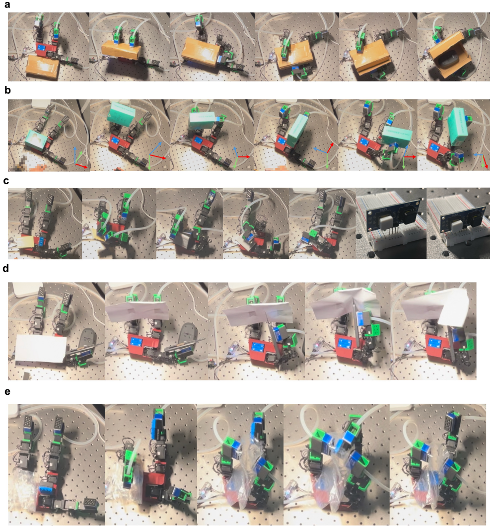
Figure 2: S-Leap Hand performing challenging in-hand manipulation. a. Opening a packed box. b. In-hand re-orientation. c. In-hand breadboard insertion. d. Paper cutting. e. Opening a plastic bag and put an object inside it.
