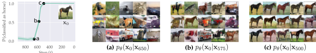
Figure 3: Specific features appearing at specific steps. (Left) For a given image of a horse ( \mathbf{x}_0 ) generated by a CIFAR-10 DDPM model, we plot the likelihood that samples from the distribution p_\theta(\cdot|\mathbf{x}_t) (see Section 2) are classified as a horse according to a CIFAR-10 classifier. This likelihood increases rapidly around steps 650 to 500, suggesting that these steps are most responsible for the formation of this feature. (Top) For three steps t in this range, we visualize samples from p_\theta(\cdot|\mathbf{x}_t) . (Bottom) At each of these steps, we also visualize the training examples with the highest influence (positive in green, negative in red) identified by our method. Note that once the “horse” feature begins to appear (around t = 575 ), positive influencers begin to reflect it. However, after this feature is “decided” (around t = 500 ), negative influencers also begin to reflect it.
