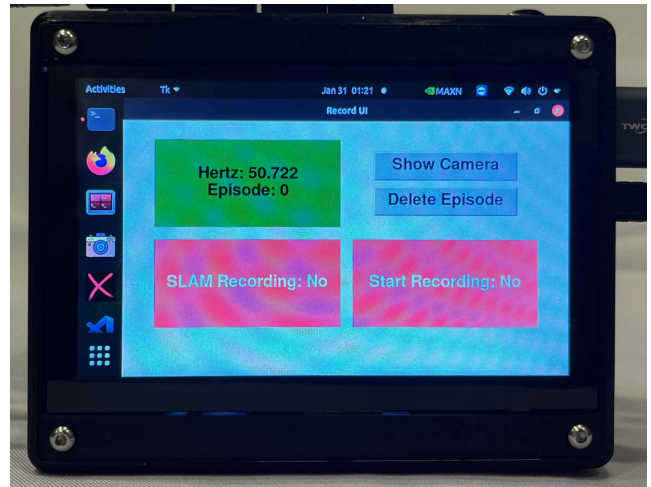
Fig. 7: DexWild-System features a simple and easy-to-use interface for deployment by untrained data collectors.
